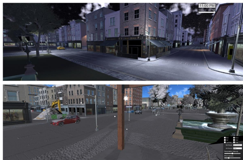
Figure 2. (Top): User can manipulate the time of the day via the time slider. Changing time affects how the environment looks and sounds due to the change in people and traffic in the city square, based off the behaviour settings of each sound source. Cities are dynamically lit after sundown. (Bottom): A weather module can help plan for different contexts, including seasons and weather conditions like precipitation, cloud coverage, and wind intensity. By changing to winter, snow is dynamically added to surfaces and the daylight hours will change due to the sun cycle changing with time of year, in respect to the city's selectable latitude and longitude.
