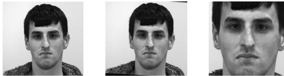
Figure 3. Face alignment and cropping. From left to right: original image, face aligned image, cropped image.
