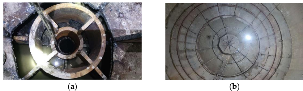
Figure 6. Homogeneous pulp-making equipment; (a) Section of the lower sand mouth and (b) Slurry ring pipe.
