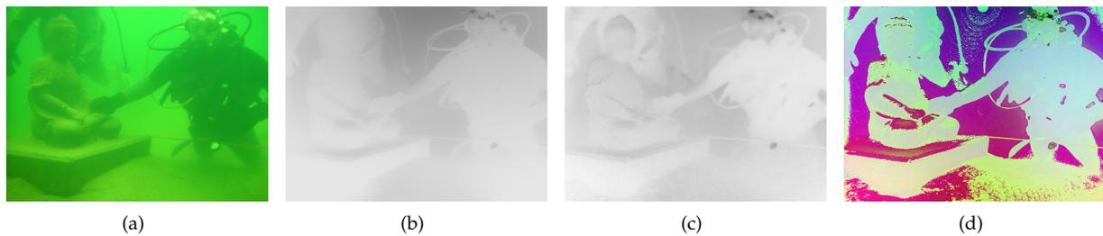
**Figure 1.** (a) An underwater image; (b) transmission map estimated by UDCP; (c) transmission map estimated by LDCP; (d) transmission map estimated by the proposed algorithm.
