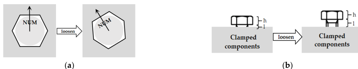
Figure 1. Two categories of bolt loosening detection. (a) Relative rotation recognition; (b) Relative length recognition.
