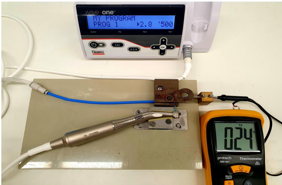
Figure 1. VB instrument set up with a cyclic fatigue rig with a thermocouple for tracking the temperature.
