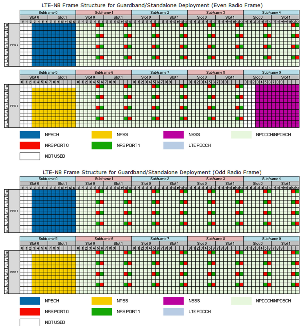
Figure 4. Allocation scheme of channels and signals in even frames (up) and odd frames (down) in guard-band and stand-alone mode [32].
