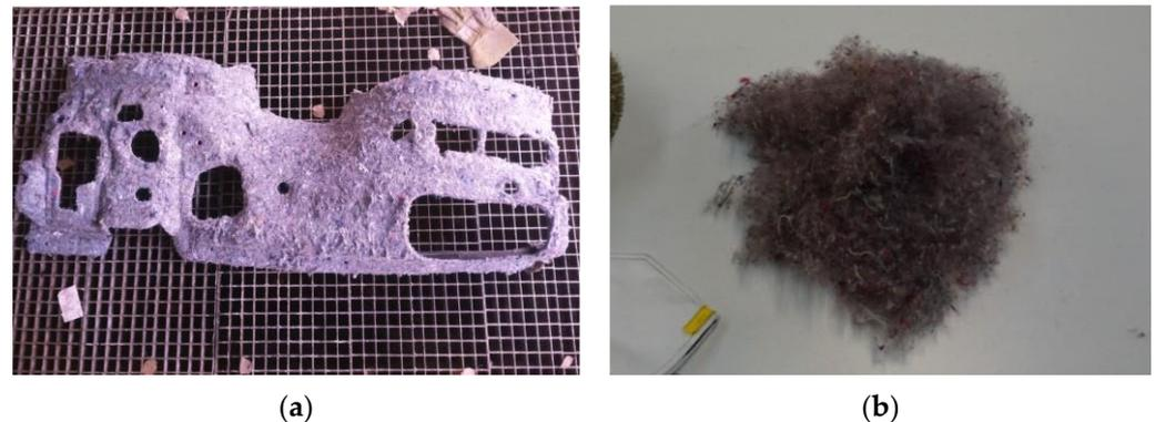
**Figure 1.** Waste felt materials from the automotive industry, (a) in the form of soundproofing boards, (b) after shredding.
