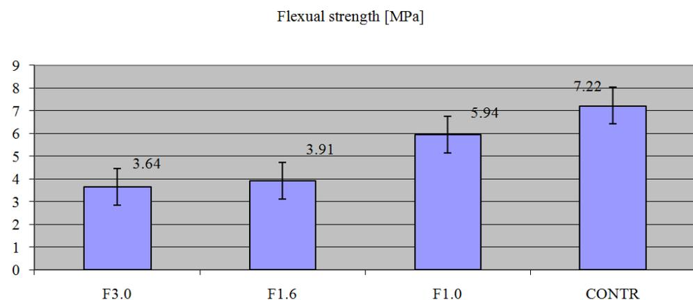
**Figure 6.** Results of tests on the tensile strength of composites by bending in a three-point scheme.
