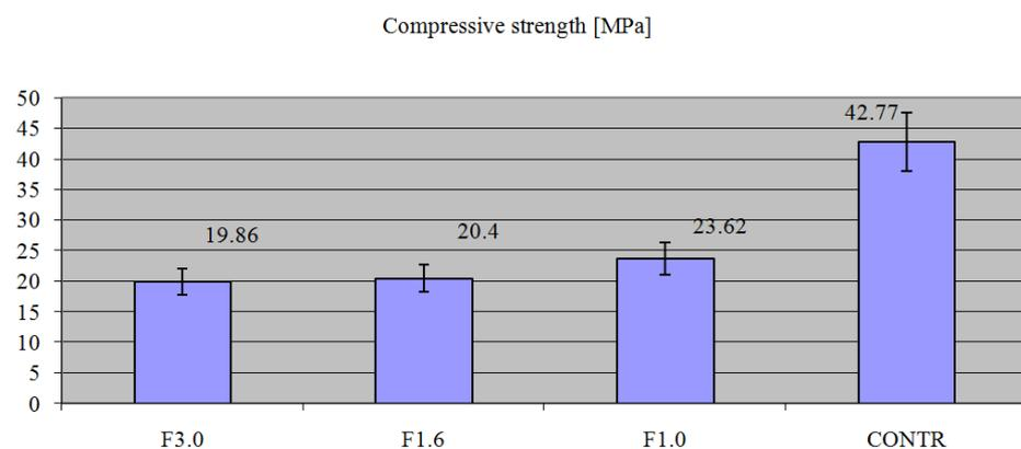
Figure 5. Compressive strength results of the composites.
