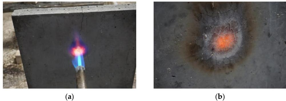
**Figure 8.** Damage to insulation boards that occurred during the temperature analyses carried out. (a) cracking of CONTR board, (b) peeling of F3.0 composite.
