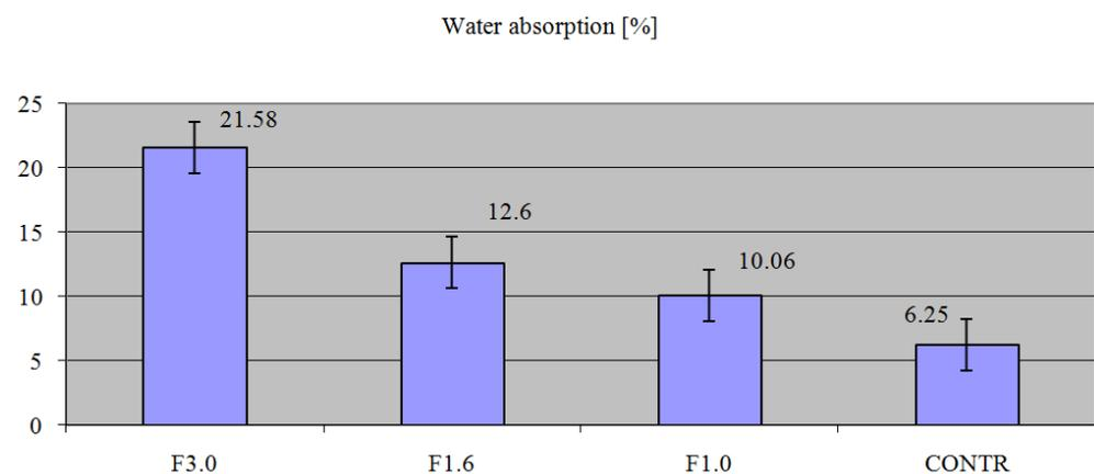
Figure 4. Results of the saturation test of the composites.
