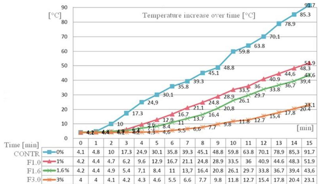
Figure 7. Data obtained during the exposure of the hot air jet to insulation boards made of composites.
