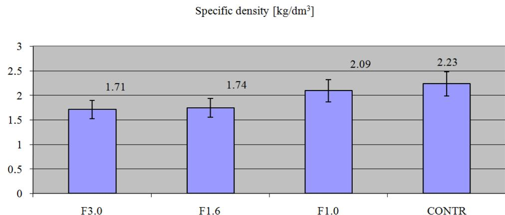
**Figure 3.** Results of specific density testing of composites.
