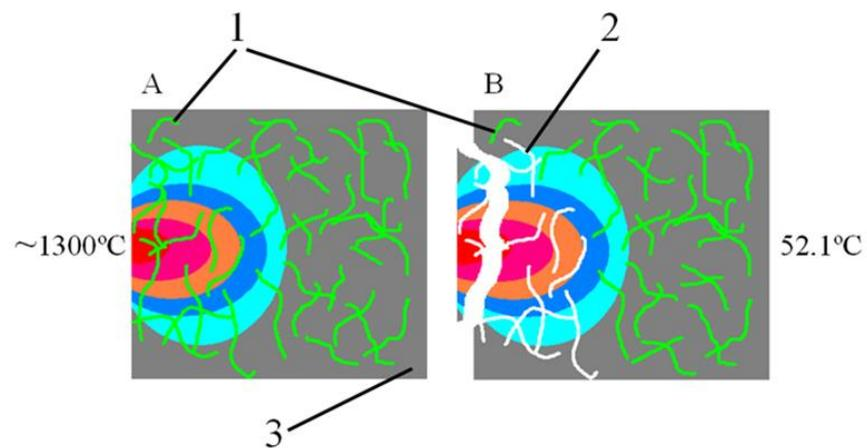
**Figure 11.** Hypothetical temperature distribution and surface failure pattern of F3.0 composite specimens. 1—recycled fibres in the composite, 2—voids formed after melting of fibres due to high temperature, 3—cement stone. The colours indicate the temperature propagation within the composite (A—high temperature interaction phase. B—superficial destruction of the composite).
