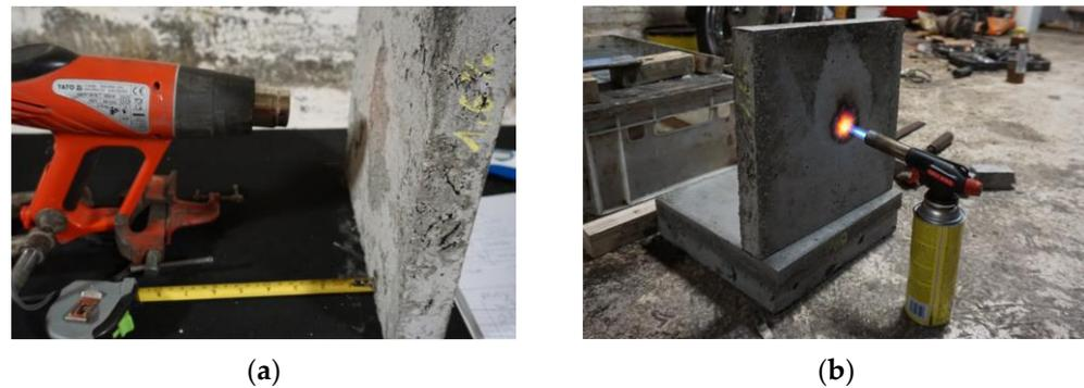
**Figure 2.** Temperature tests. (a) Test stand for the insulation test of the samples. (b) Test stand for the author's fire resistance test.
