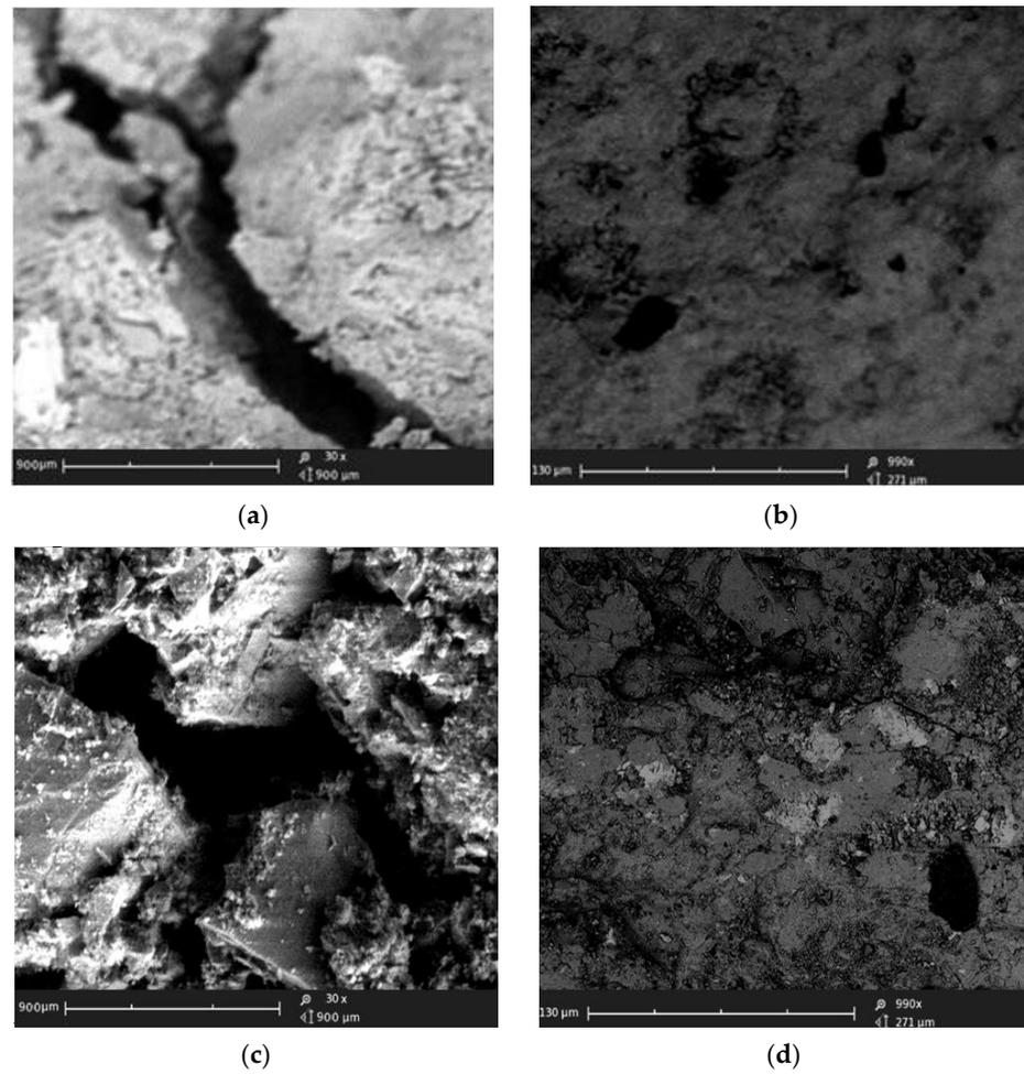
**Figure 10.** Damage to the structure of the F3.0 composite as a result of fire, (a,c)—pronounced cracks in the structure, (b,d)—void after fibre melting.
