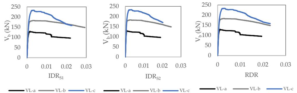
**Figure 5.** PO curves obtained for VL-a, VL-b, and VL-c. The three plots report the IDR of the first level (left), the IDR of the second level (centre), and the RDR (right) of the masonry wall.
