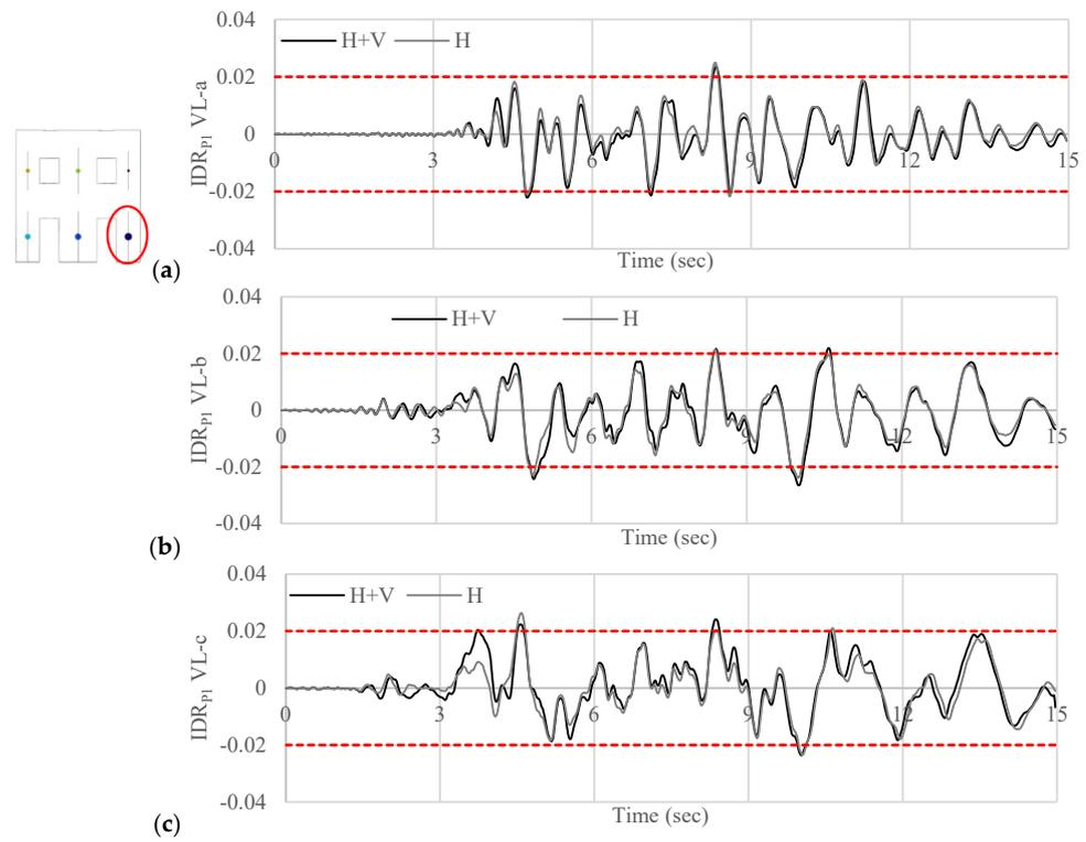
**Figure 12.** IDRs obtained subjecting the structure with VL-a (a), VL-b (b), and VL-c (c) to earthquake #1. The red lines indicate the IDR limit of 2%.
