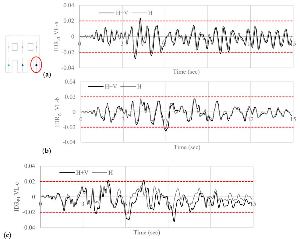
**Figure 13.** IDRs obtained subjecting the structure with VL-a (a), VL-b (b), and VL-c (c) to earthquake #2. The red lines indicate the IDR limit of 2%.
