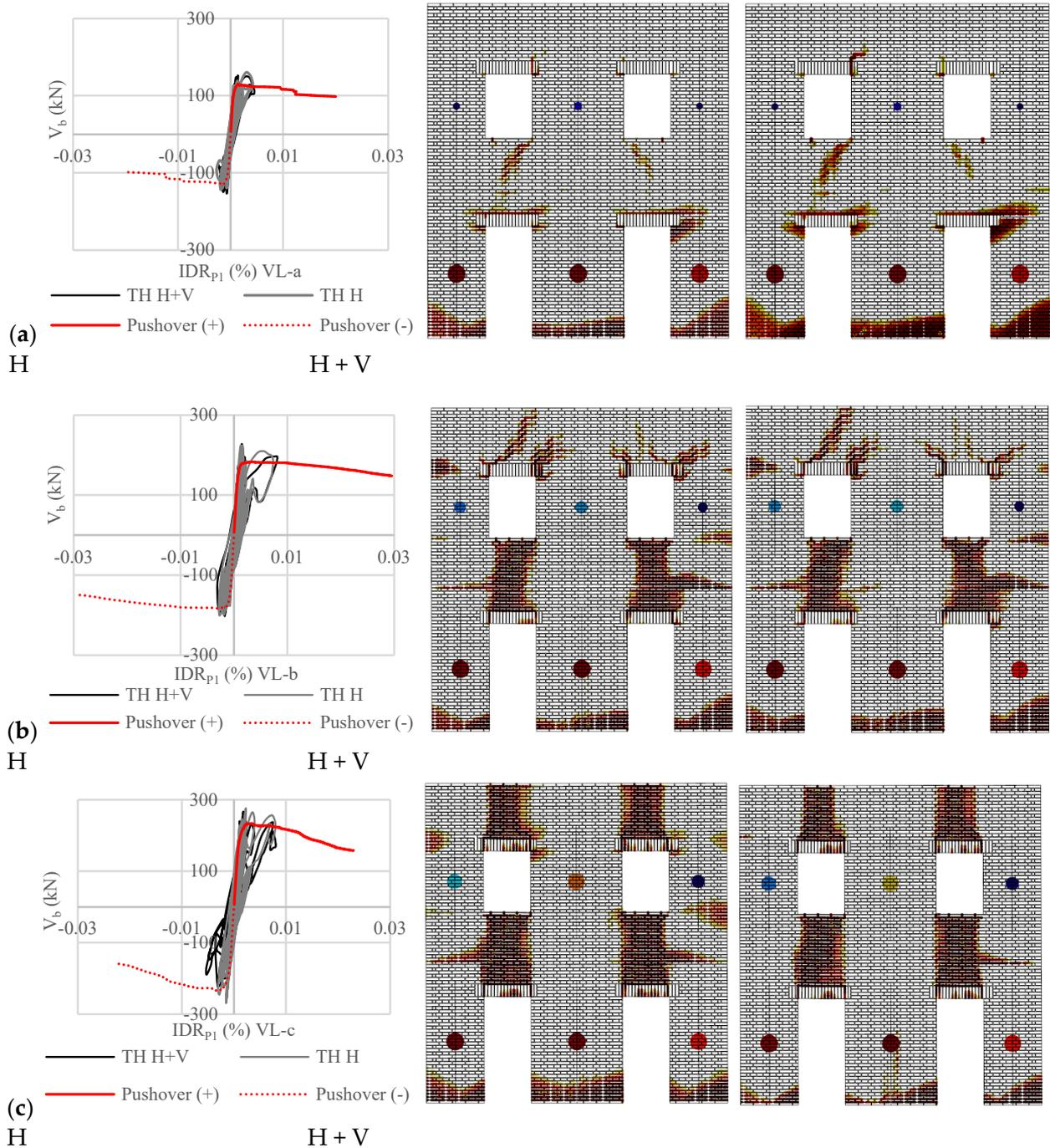
**Figure 17.** IDR- $V_b$  curves and crack patterns obtained for the earthquake #1. TH results for the H component are in grey, TH results for H + V components are in black, the PO curve for positive displacements is the continuous red line, and the PO curve for negative displacements is the dashed red line. Loading conditions: VL-a (a), VL-b (b), and VL-c (c).
