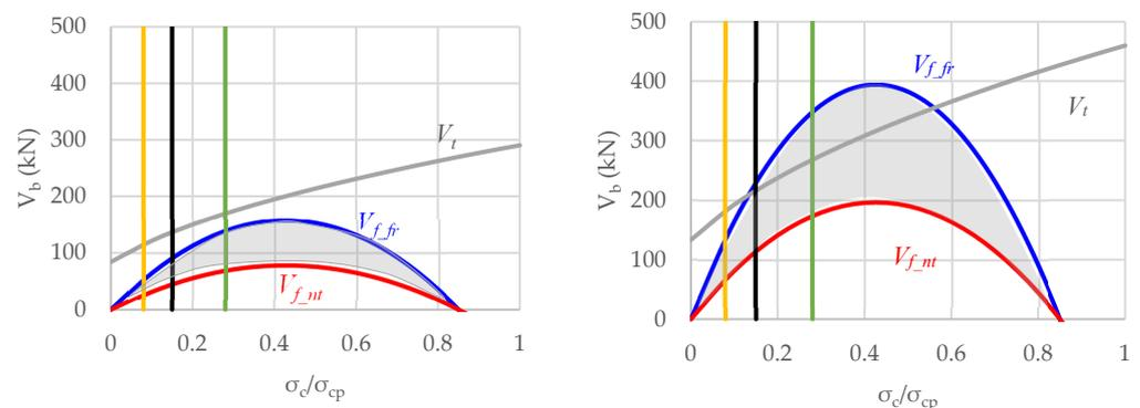
**Figure 4.** Resistance domains of masonry piers P1 (left) and P2 (right). Vertical lines correspond to VL-a (yellow line), VL-b (black line), and VL-c (green line). Grey lines correspond to the shear capacity  $V_t$ , and the red and blue curves refer to flexural capacities corresponding to free rotation ( $V_{f\_fr}$ ) or absence of rotation at the top of the panel ( $V_{f\_nr}$ ), respectively.
