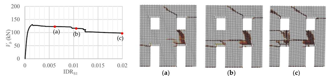
**Figure 6.** Cracking pattern of the masonry wall with VL-a. From left to right, damage scenarios corresponding to (a) 0.5%, 1% (b), and 2% (c) of  $IDR_{S1}$ .
