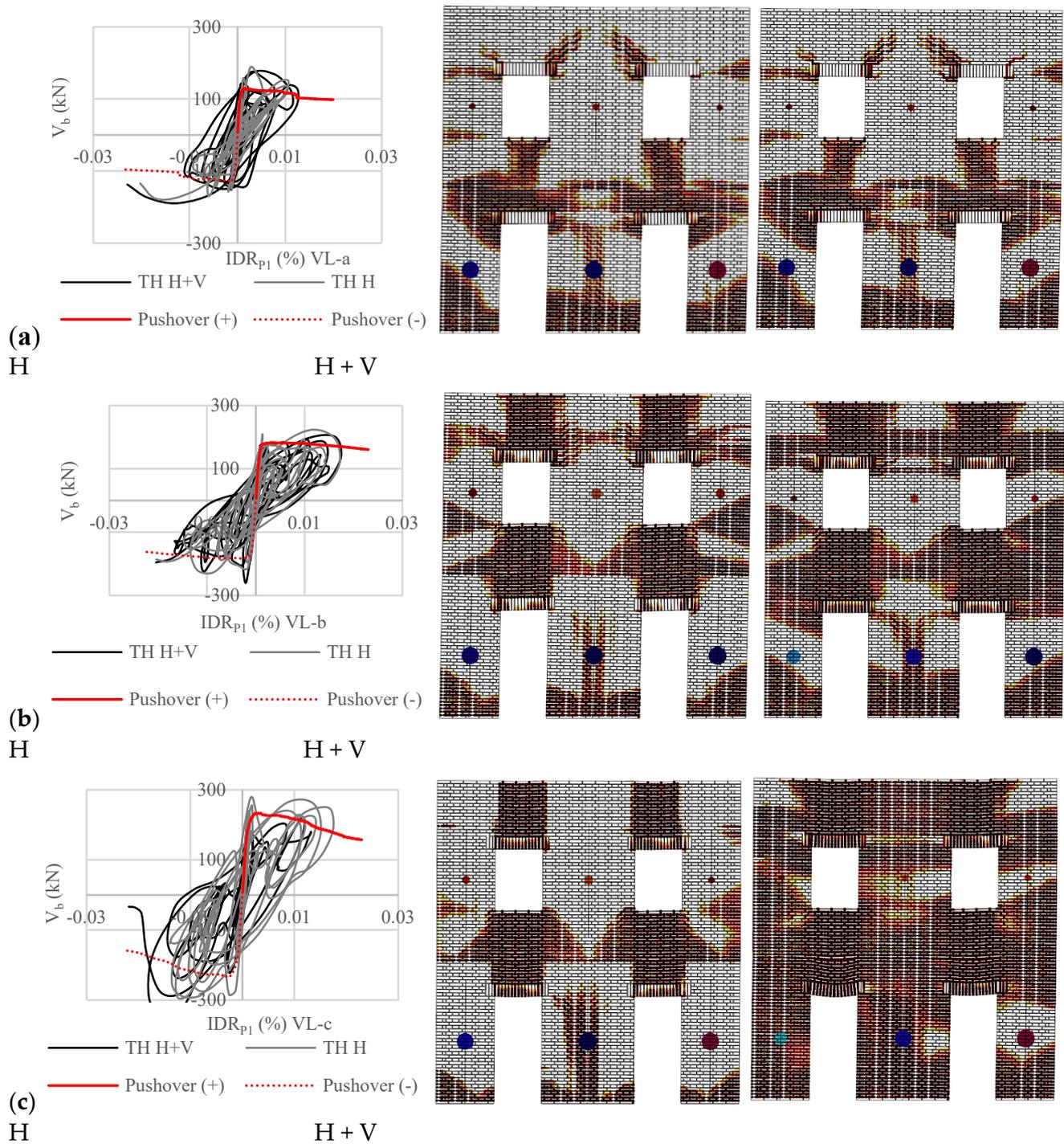
**Figure 16.** IDR- $V_b$  curves and crack patterns obtained for earthquake #2. TH results for the H component are in grey, TH results for H + V components are in black, the PO curve for positive displacements is the continuous red line, and the PO curve for negative displacements is the dashed red line. Loading conditions: VL-a (a), VL-b (b), and VL-c (c).
