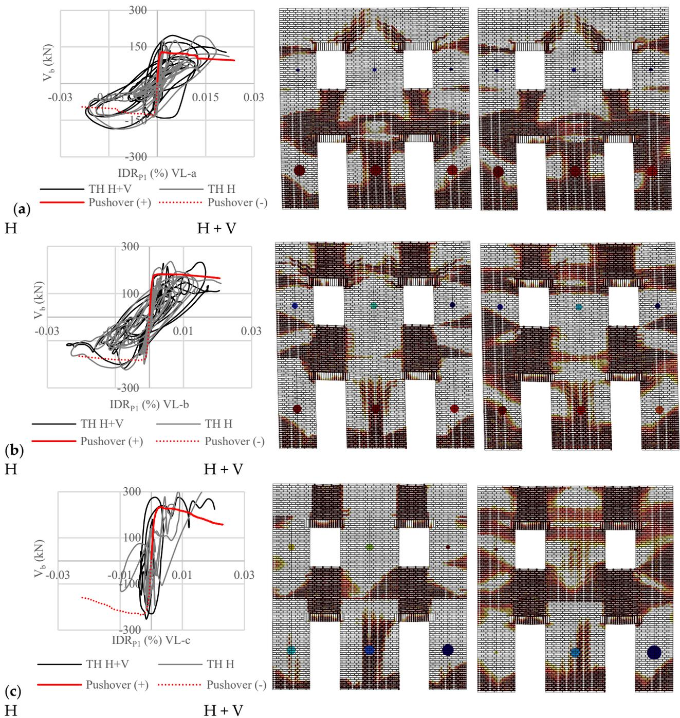
**Figure 15.** IDR- $V_b$  curves and crack patterns obtained for earthquake #1. TH results for the H component are in grey, TH results for H + V components are in black, the PO curve for positive displacements is the continuous red line, and the PO curve for negative displacements is the dashed red line. Loading conditions: VL-a (a), VL-b (b), and VL-c (c).
