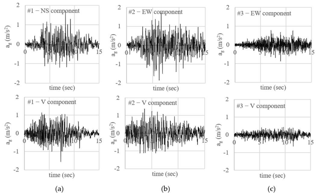
**Figure 9.** Horizontal (top row) and vertical (bottom row) recorded accelerograms: (a) earthquake #1, Norcia 30 October 2016, 14.9 km from the epicentre; (b) #2 Norcia 30 October 2016, 19.2 km from the epicentre; and (c) #3 Norcia 30 October 2016, 20 km from the epicentre.
