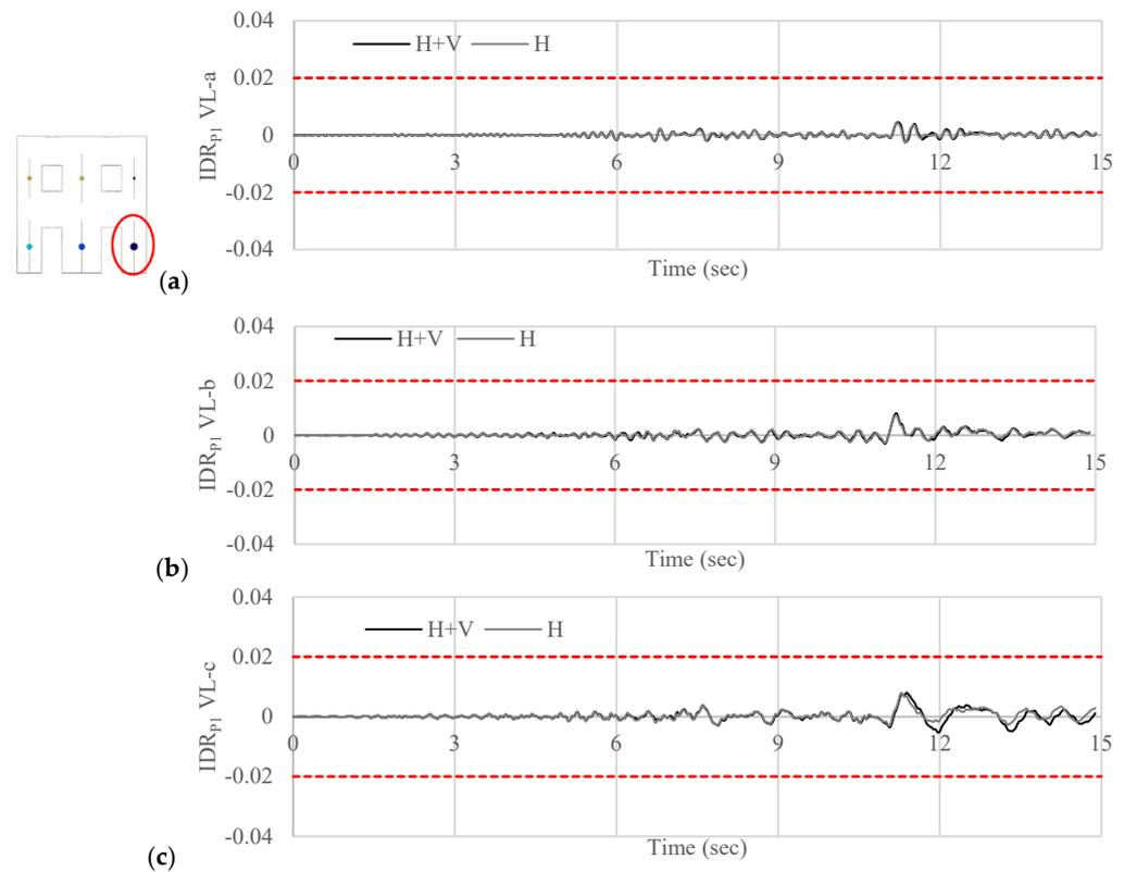
**Figure 14.** IDRs obtained subjecting the structure with VL-a (a), VL-b (b), and VL-c (c) to earthquake #3. The red lines indicate the IDR limit of 2%.
