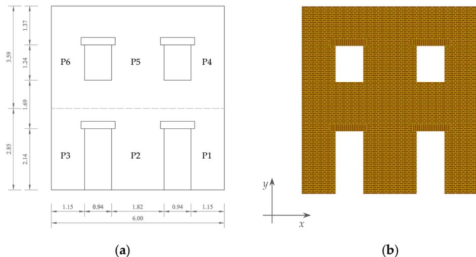
**Figure 3.** Wall geometry: (a) element dimensions (m), numbering of masonry piers, and (b) layout of the numerical model.
