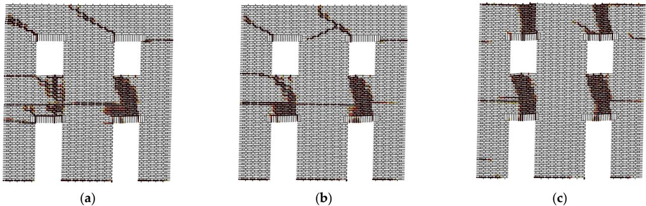
**Figure 7.** Crack pattern of the masonry wall corresponding to an IDR of the first level equal to 2% for (a) VL-a, (b) VL-b, and (c) VL-c.
