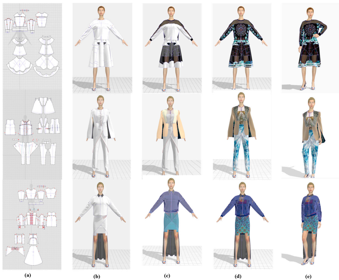
Figure 6. Digital clothes applied to an avatar model in steps: (a) creating a pattern, (b) fitting to the avatar, (c) shading and coloring the fabric properties, (d) mapping the texture on the clothing, and (e) posing the avatar.
