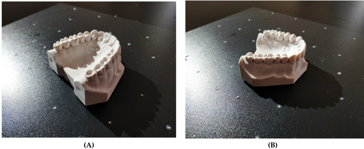
Figure 3. (A) Model manufactured through SLA; (B) Model manufactured through DLP.
