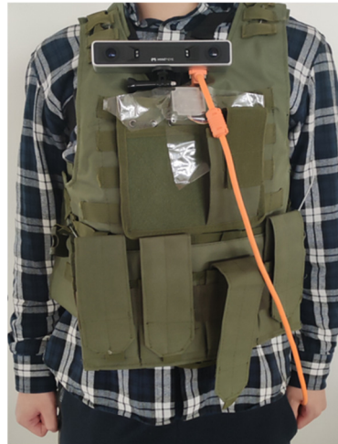
Figure 4. Data Acquisition. The IMU data collected on the wearable are the training set, and the data collected by the camera device are the ground truth information.
