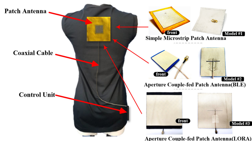
Figure 1. Illustrated view of fabric-based antennas integrated into fabric clothing.
