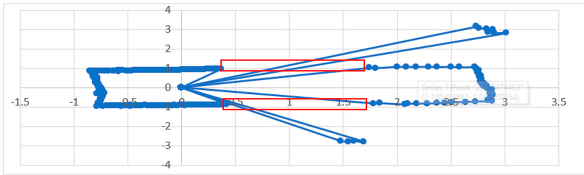
Figure 18. The 360 range mapping laser scan points mapped radially around the robot. The red boxes show the locations of side mirrors.
