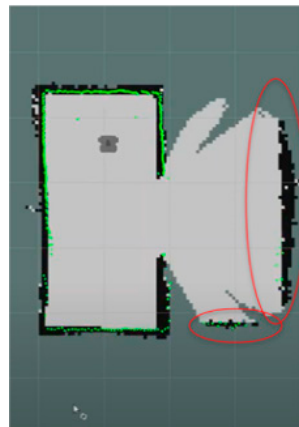
Figure 14. Observation of the reflected boundary detected behind the surface of the mirror.
