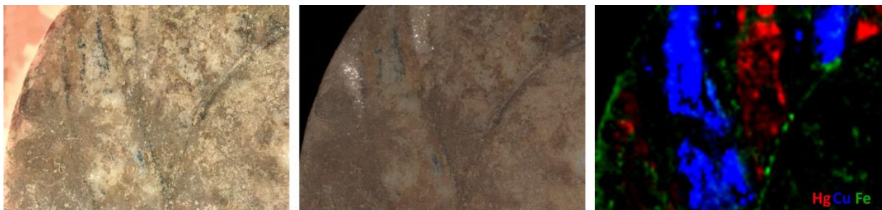
Figure 6. Composite elemental maps of Cu, Fe, and Hg showing the distribution of the corresponding pigments (Cu for azurite and Egyptian blue; Hg for cinnabar) on the wing (area A of Figure 4). (left), VIS image of the scanned area; (middle), stacked VIS-VIL image; (right), XRF map.
