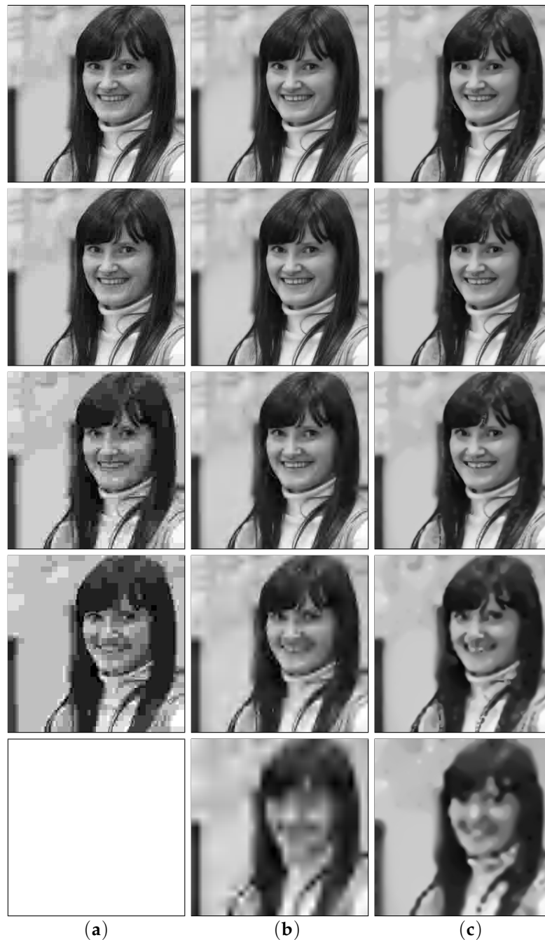
Figure 15. Comparative overview of reconstructed images for image beauty ranging from 0.8 bpp (top row) to 0.05 bpp (bottom row). Compression methods: (a) JPEG, (b) JPEG 2000, and (c) EEDC-BSSP.
