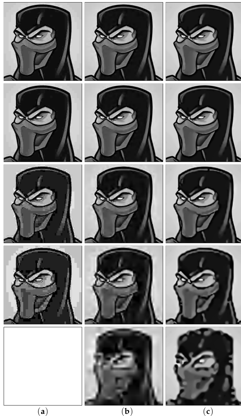
Figure 16. Comparative overview of reconstructed images for image mask ranging from 0.8 bpp (top row) to 0.05 bpp (bottom row). Compression methods: (a) JPEG, (b) JPEG 2000, and (c) EEDC-BSSP.
