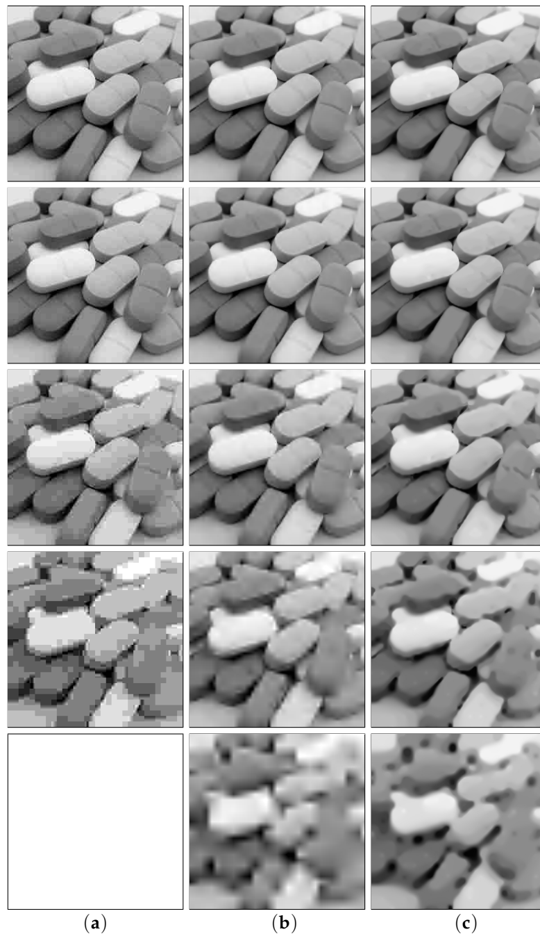
Figure 17. Comparative overview of reconstructed images for image pills ranging from 0.8 bpp (top row) to 0.05 bpp (bottom row). Compression methods: (a) JPEG, (b) JPEG 2000, and (c) EEDC-BSSP.
