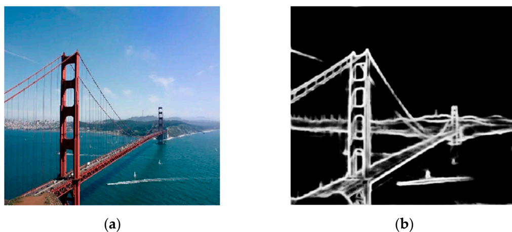
Figure 1. Edge detection results of HED network on natural images. (a) Bridge original image; (b) Bridge image HED network edge detection.
