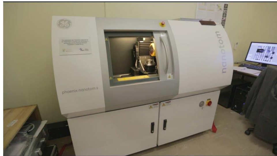
Figure 7. The General Electric Nanotom S CT scanner used to determine the porosity characteristics of the 3D printed and cast concrete in this study.
