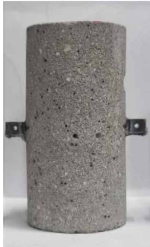
Figure 5. Test specimen with two lateral Perspex blocks attached for target marker positioning.
