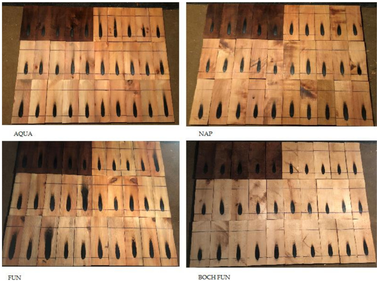
Figure 5. Presentation of wood samples after the experiment. The order of wood species is sorted from left to right as follows: 1 row—SM (spruce) and SMR (red spruce); 2 row—JAS (ash) and BOR (pine); 3 row—DUB (oak) and BUK (beech).
