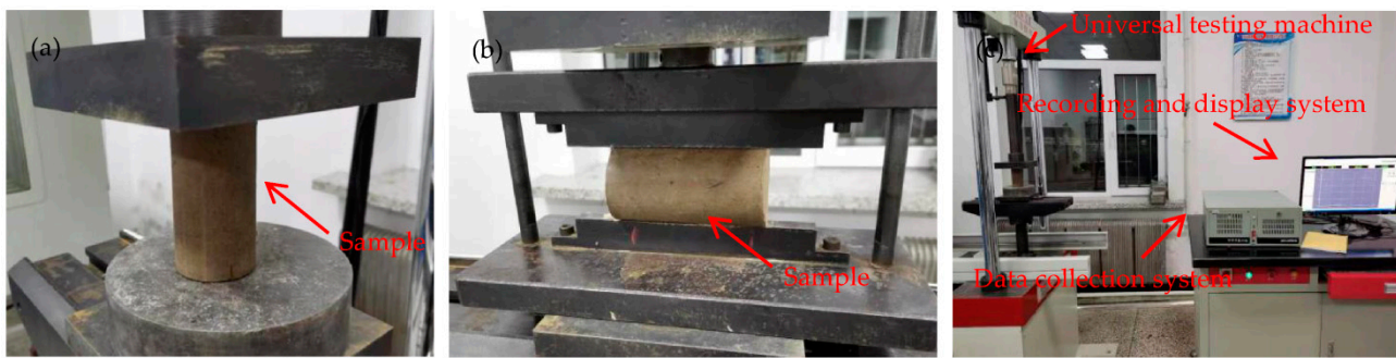
Figure 4. Universal testing machine used for tests: (a) UCS test, (b) STS test, and (c) test system.
