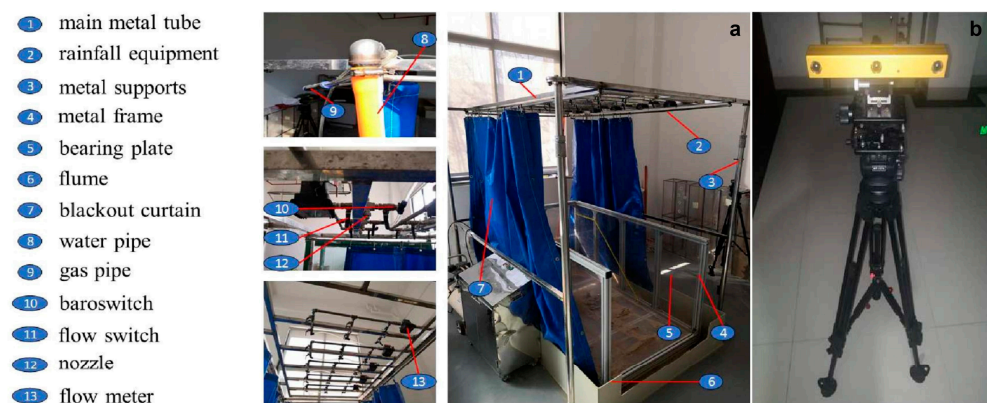
Figure 1. Physical experiment system. (a) Rainfall system and (b) trinocular stereo camera.
