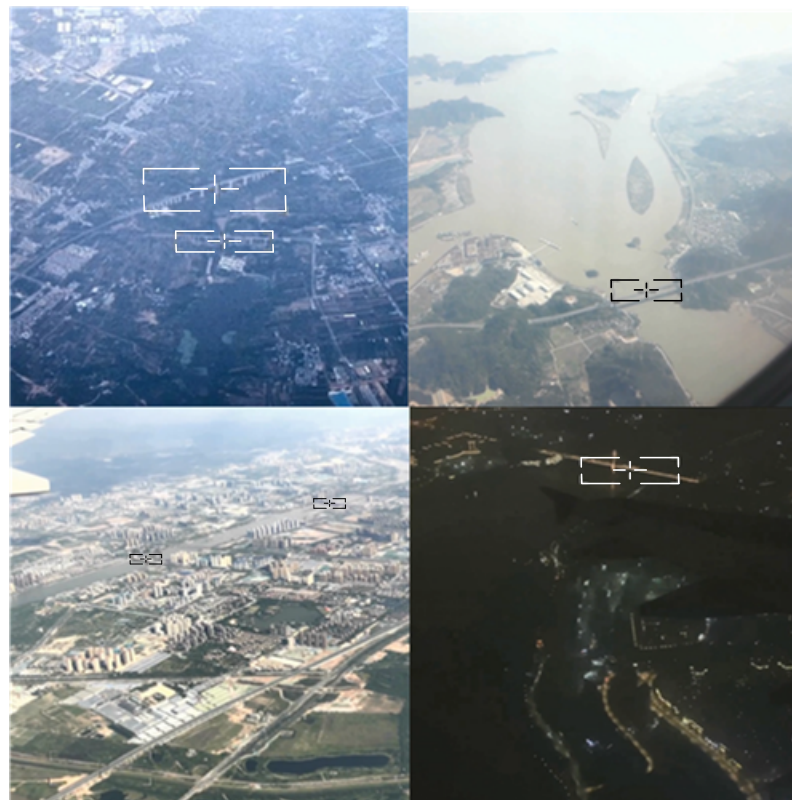
Figure 18. The actual output of the bridge detection in the aerial video using TinyYolo inference with the acceleration core.
