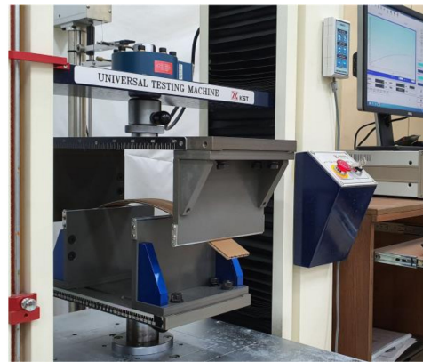
Figure 4. Four-point bending test apparatus for the corrugated fiberboard specimen.
