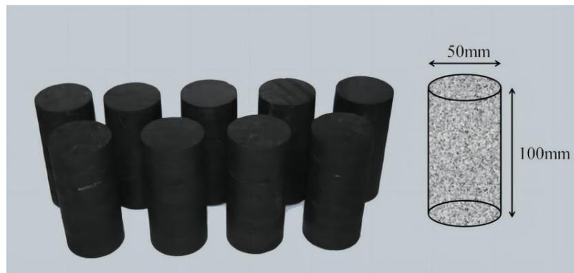
**Figure 1.** Partial test coal specimens after processing.
