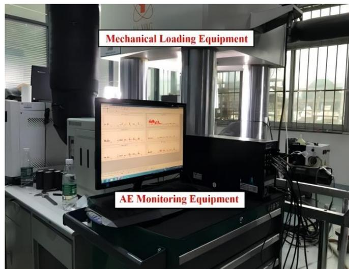
**Figure 2.** Mechanical loading equipment and AE system.
