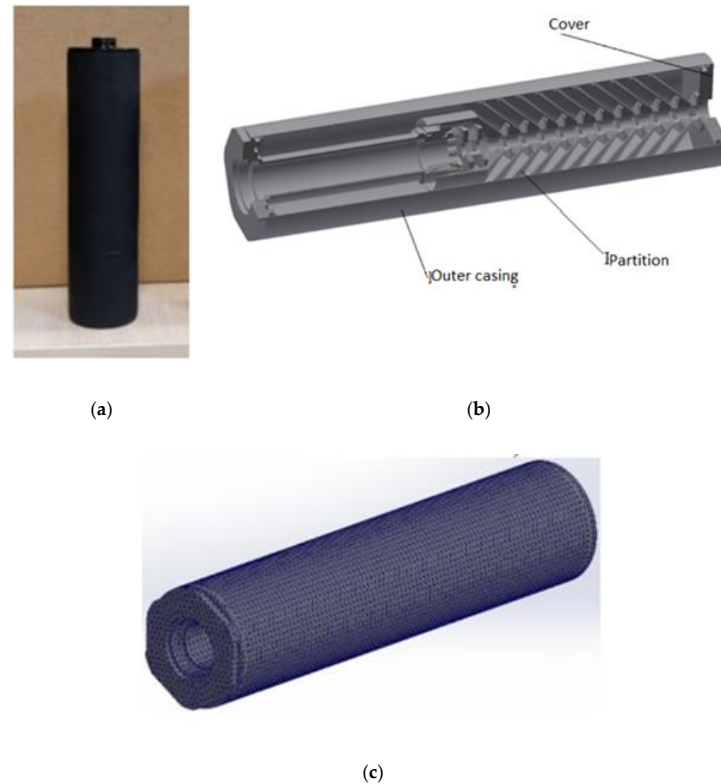
Figure 1. The total view (a), 3D model (b) and the silencer finite element grid (c).
