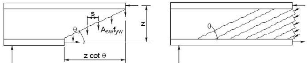
Figure 8. Location of the inclined struts [41].
