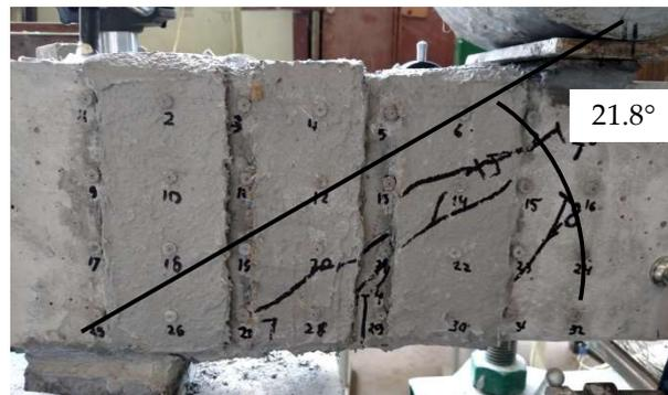
Figure 9. The angle of inclined struts in the sample BS 1.1.1-0.
