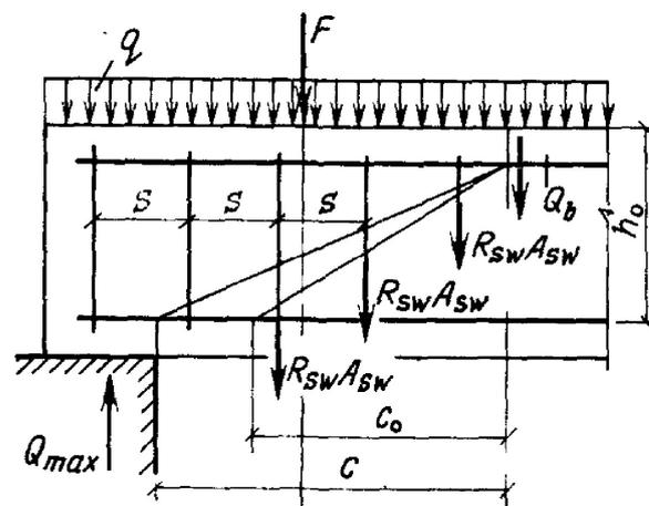
**Figure 3.** Scheme of the shear forces when calculating according to the engineering method [38].
