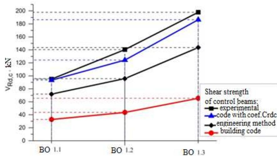
**Figure 6.** Experimental and theoretical data of the shear strength for control samples.
