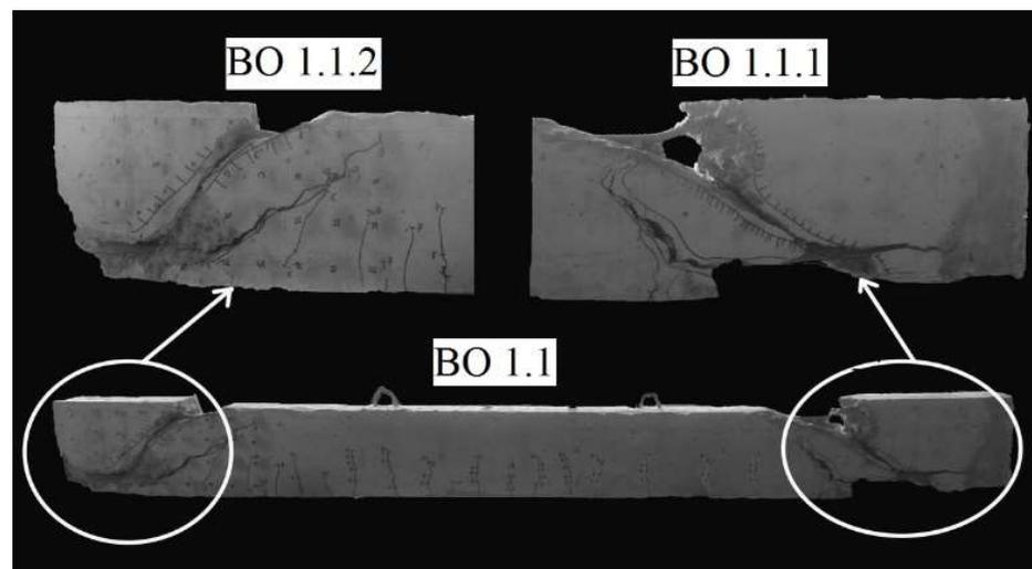
**Figure 1.** Tested control samples without internal shear reinforcement.
