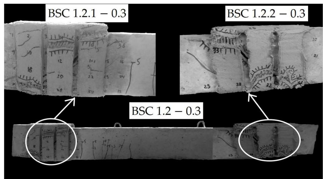
**Figure 2.** General view of exhausted shear strength of reinforced samples.
