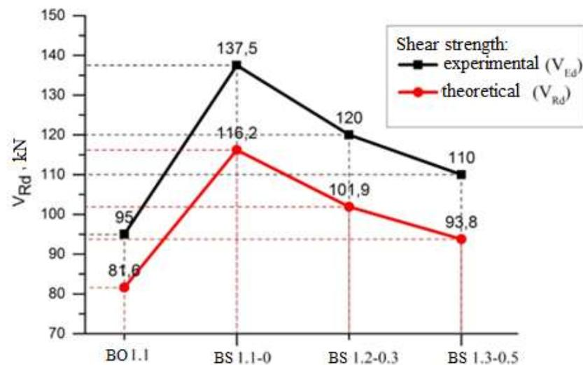
**Figure 10.** Comparison theoretical and experimental results of shear strength of strengthened beams.
