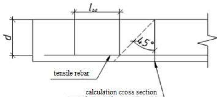
Figure 4. A model of the influencing factors on the shear strength of a support area [2,3].
