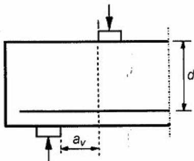
Figure 5. Case of applying load for the coefficient  $\beta$  [2,3].
