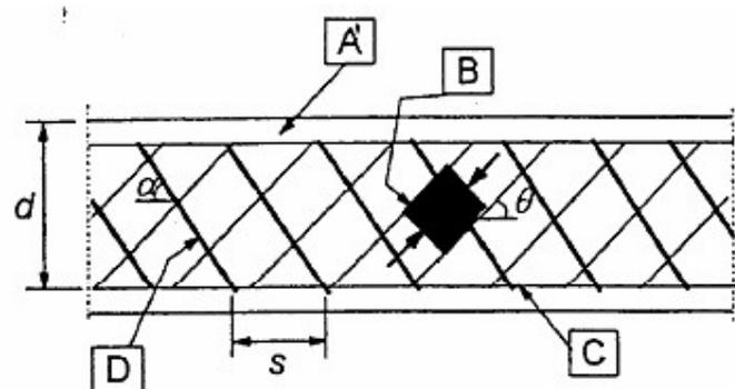
**Figure 7.** Truss model of the calculation state in the supporting area of RC beam [2]: A—compressed chord; B—compressed struts; C—tensile truss chord; D—tensile struts.
