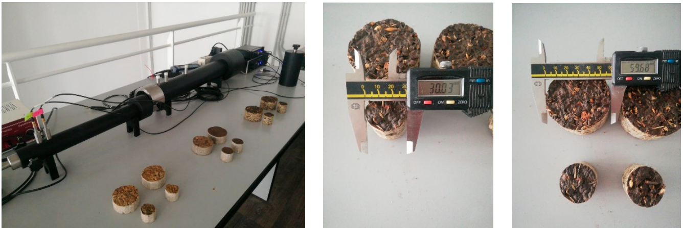
Figure 2. The normal incidence sound absorption coefficient measurement set-up and specimen sizes.
