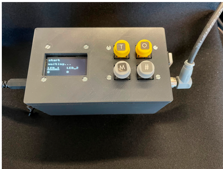
Figure A7. Controller unit with tactile buttons, ON/OFF switch, OLED display, power supply, and power output. Buttons are used for switching between the modes (Button M: start, constant, and day/night) and the LED rows (Button #: Row 1 and Row 2). The other two buttons are counters for fast and precise adjustment of the light intensity. The first counter increases intensity in 10% steps (Button T). The second increases intensity in 1% steps (Button O).
