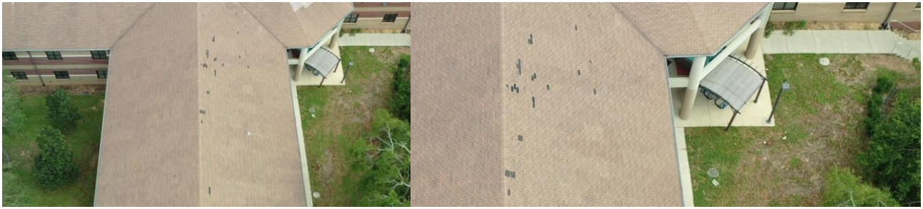
Figure 2. Examples of the positive damage images for the CC approach.
