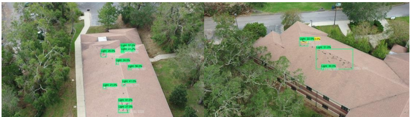
Figure 8. Example results using the CNN approach. The images depict frames from aerial footage from Argo Hall and Martin Hall. The CNN detects damages with green squares (light damage) and a yellow square (medium damage), with confidence ratings and the pixel locations.
