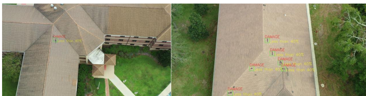
Figure 5. Example results obtained using the CC approach.
