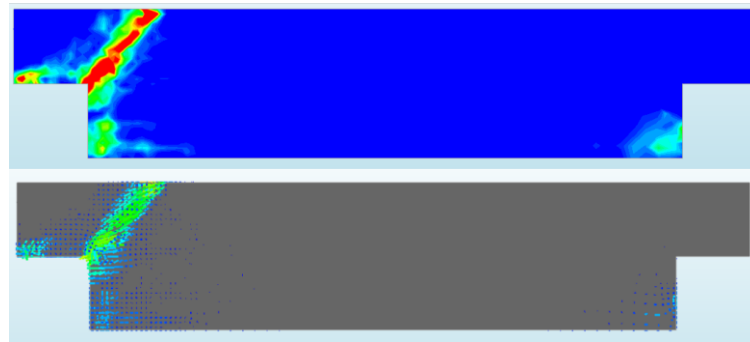
Figure 22. Principal strains and cracking in the numerical model for the analysis of prestressing's impact on bearing capacity.
