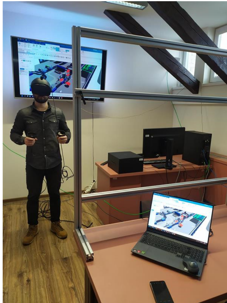
Figure 4. Linking TX Plant Simulation with VR via the Go VR function.
