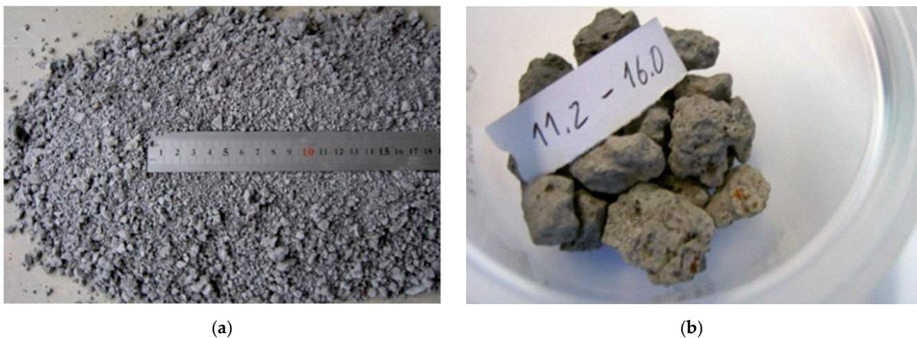
Figure 2. Particles of SSA: (a) fraction 0/20; (b) fraction 11.2/16.0.
