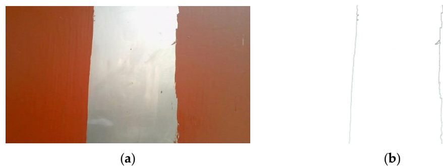
Figure 11. Process of inspecting missed painted areas: (a) image of painting to be tested; (b) Canny edge detection result.
