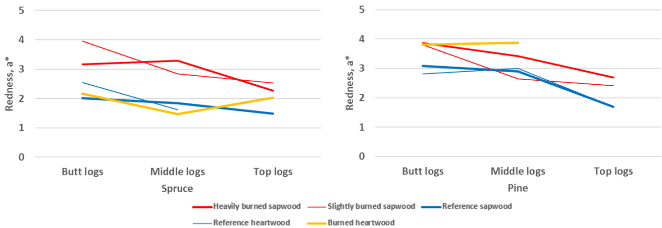
Figure 7. Redness ( a^* ) of spruce and pine wood by log type: sapwood of burned trees on the opposite sides (concerning the intensity of forest fire) and heartwood of burned trees, sapwood, and heartwood of reference trees. Moisture content is 12%.
