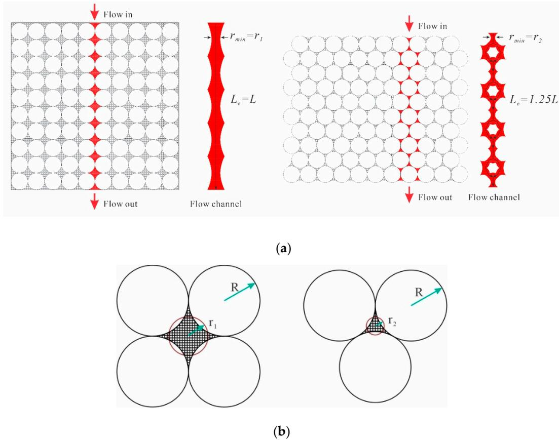
**Figure 9.** (a) Flow channels and (b) the corresponding pores of two types of particle arrangements in 3D printing techniques.
