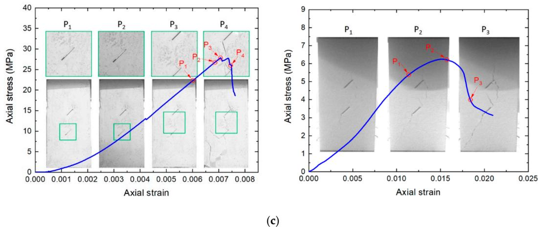
**Figure 6.** Comparison of the stress–strain curves and the corresponding cracking processes between the double-flawed moulded gypsum (left) and PP (right) specimens: (a) 45°–45°, (b) 45°–75°, and (c) 45°–105°.
