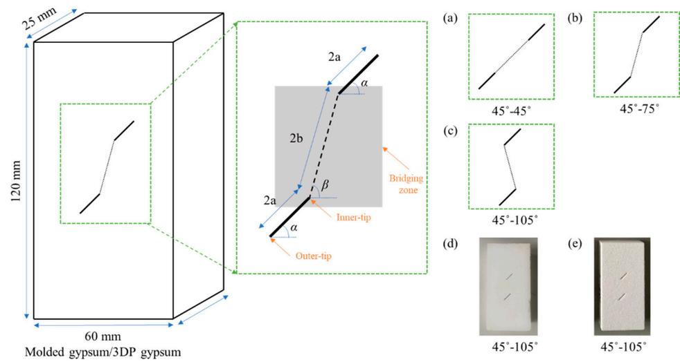
**Figure 5.** Geometry parameters defined in the present double-flaw system. (a) the geometry of flaws for sample 45°–45°; (b) the geometry of flaws for sample 45°–75°; (c) the geometry of flaws for sample 45°–105°; (d) the photo of moulded gypsum sample 45°–105°; (e) the photo of 3DP gypsum sample 45°–105°.
