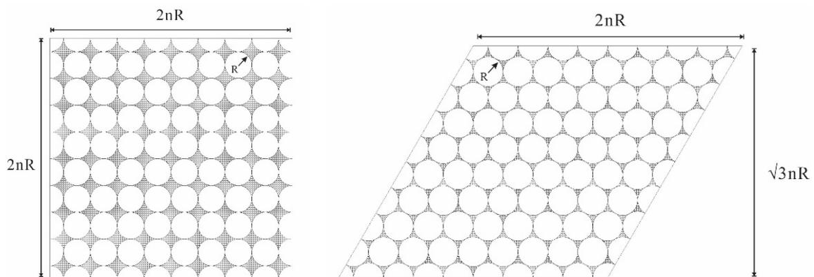
**Figure 10.** Porosity of the medium with the two types of particle arrangements.
