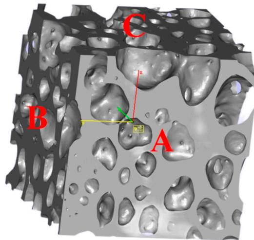
**Figure 7.** Three orthogonalized surfaces of the porous basalt in the seepage test.
