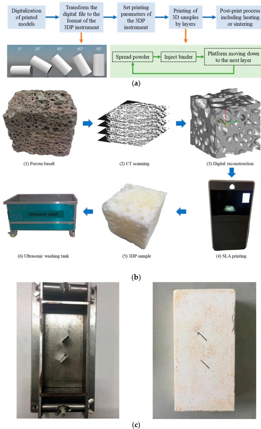
**Figure 1.** The manufacturing process of (a) plaster-based 3D printing (PP), (b) stereolithography (SLA) samples, and (c) moulded gypsum samples.
