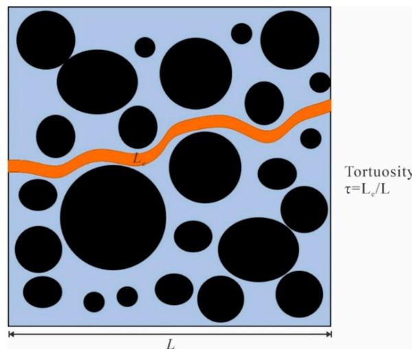
**Figure 8.** Sketch of the actual flow path and the tortuosity (Black dots represent skeletons with different sizes).
