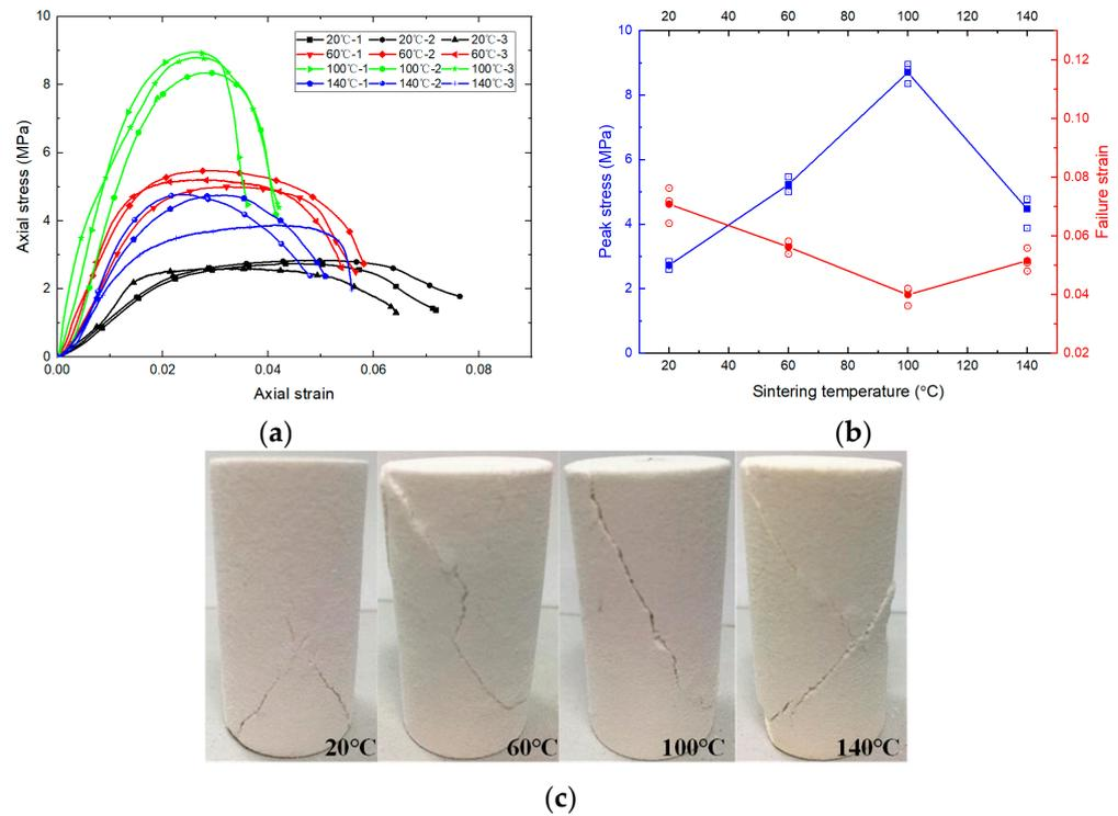
**Figure 4.** (a) Stress–strain curves and (b) peak stresses of the 3DP PP samples with different sintering temperatures (solid point—average value of each group), and (c) their failure modes.
