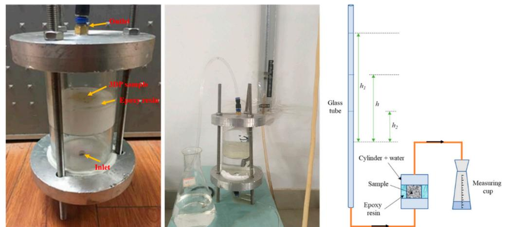
**Figure 2.** Experimental seepage test and the schematic drawing in the present study.
