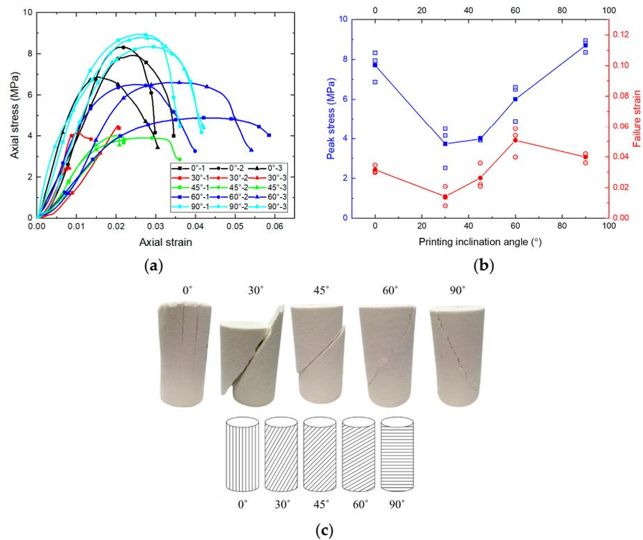
**Figure 3.** (a) Stress–strain curves and (b) peak stresses of the 3DP PP samples with different printing inclination angles (solid point—average value of each group), and (c) their failure modes.
