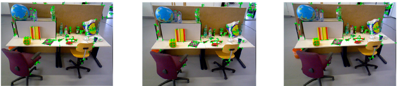
Figure 5. Extraction of the orb feature points (from left to right: Frame 1, Frame 2, and Frame 3).
