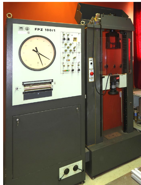
Figure 2. Typical form of the HECKERT FPZ 100/1 universal testing machine.
