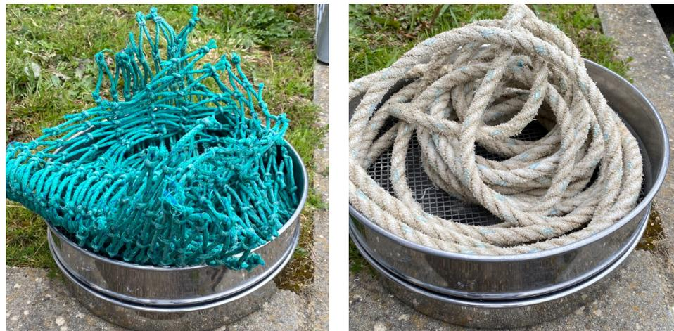
**Figure 4.** Experimental setup to collect rainwater that passed through the WFT and WFR.
