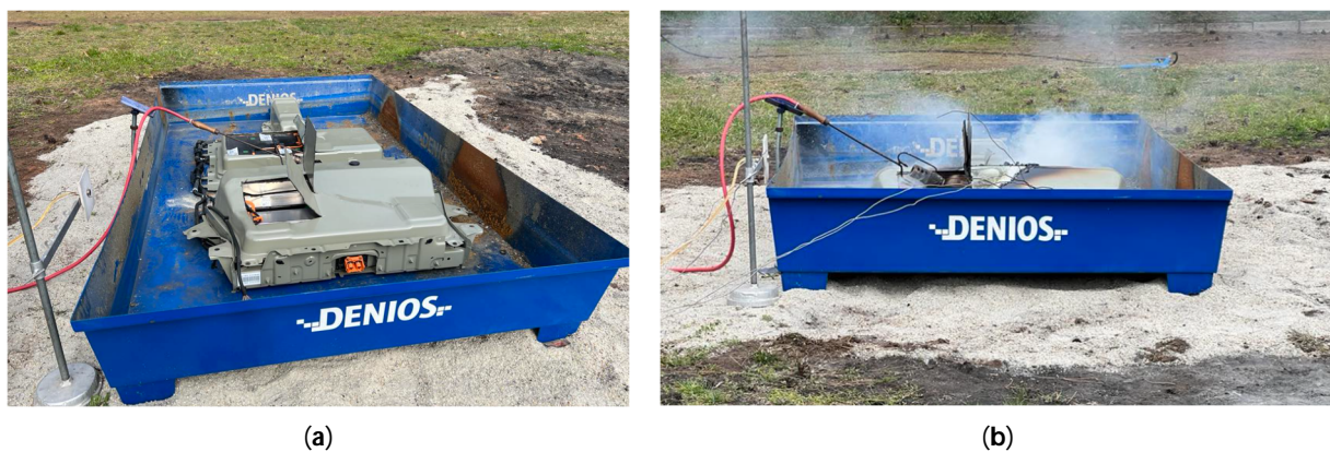
Figure 3. Experiment preview: (a) Time 0 s, inserting the external initiator into the damaged cover of the EV traction battery; (b) real experimental time 1500 s (25 min), action of the external flame.
