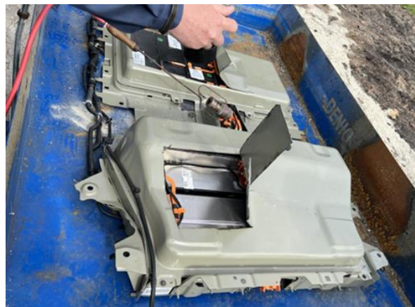
Figure 2. Scheme: The top view of the BEV placement with the location of the indicated thermocouples. (a) First gap and the location of the red and blue thermocouples; (b) second gap and the location of the blue and green thermocouples; and (c) showing the position of the thermocouples and (d) the mechanical damage of the BEV.
