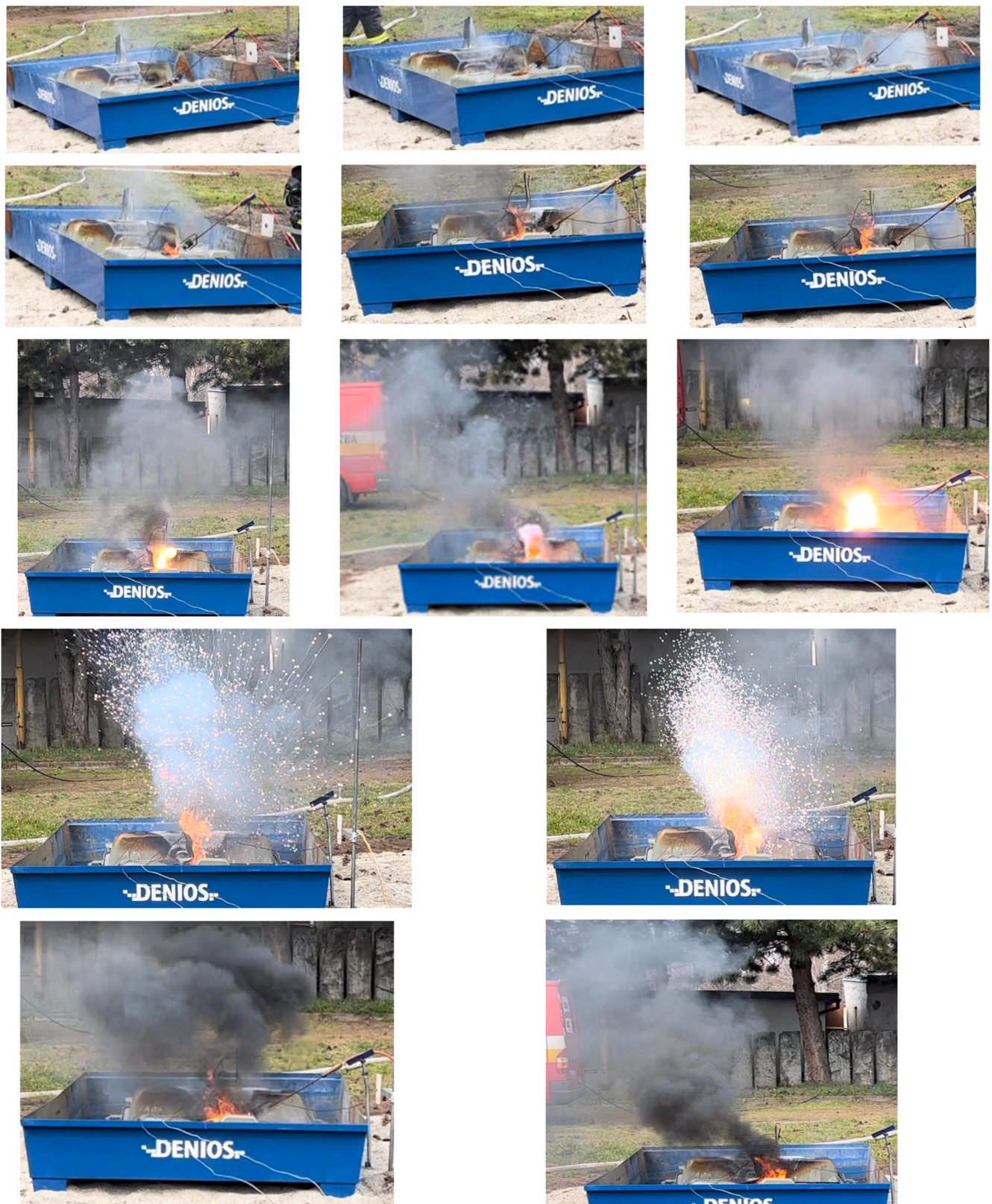
Figure 9. Photo documentation of the EV traction battery fire in Test 2 in the two-minute interval within a time frame from 180 s to 300 s. The first nine images are a cross-section of the first minute, and the remaining four images represent 25 s of the sequence in the second minute.
