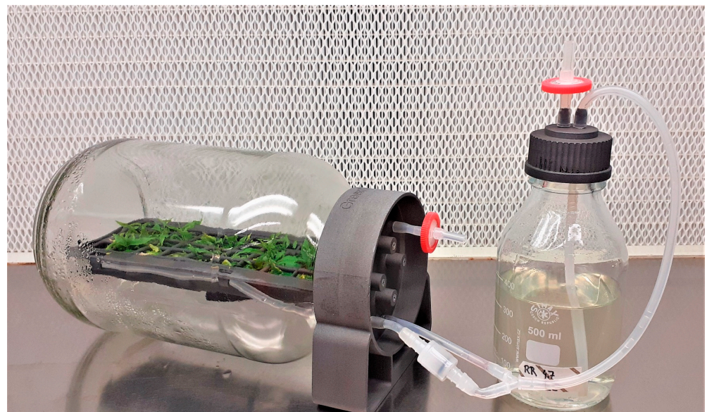
Figure 2. Assembled GreenTray®, sterilized and ready for the cultivation of plants.
