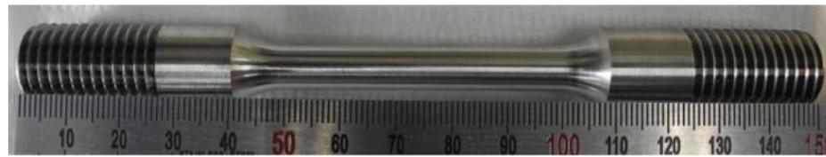
**Figure 6.** Type of round tensile test specimen.
