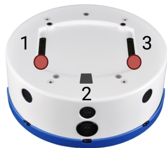
Figure 6. Keypoints the Khepera. Number 1 indicates the left marker, number 2 indicates the front marker, and number 3 indicates the right marker. These markers are used to calculate the robot's (x, y) coordinates and angular orientation through pose estimation tasks performed by the YOLO v8 model.
