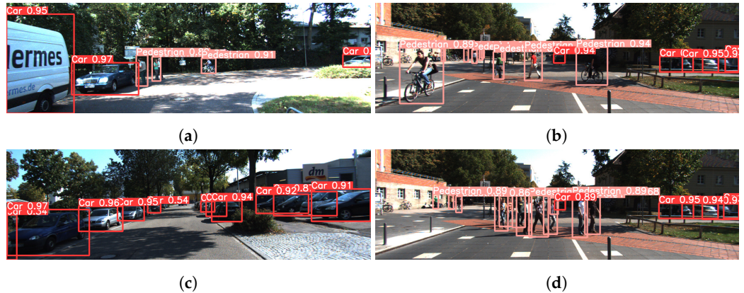
Figure 11. Detection results with EMA integration. (a) Close-up view. Detection results of large targets in close-up scenarios. (b) Distant view. Detection results of small targets in distant scenarios. (c) Car-dominant image. This image predominantly contains cars, with only a few instances not being detected. (d) Pedestrian-dominant image. All instances of pedestrians in this image are successfully detected.
