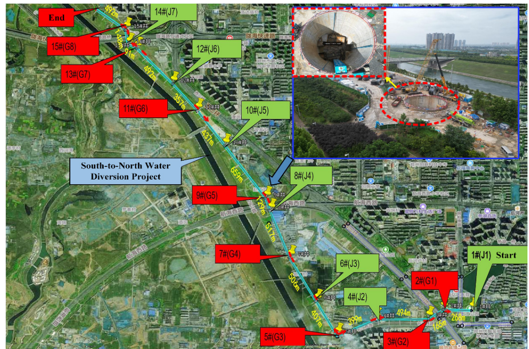
Figure 1. Caisson alignment along the Jinshui River.
