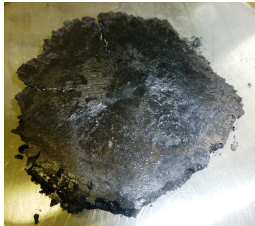
Figure 8. Example of strengthened core of test specimen residue with slenderness ratio 6.25.
