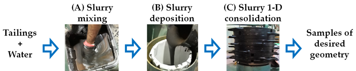
Figure 3. Slurry-based reconstitution method used to prepare the iron ore tailings samples, involving the following stages: (A) slurry uniformization through hand mixing at the desired water content; (B) the deposition of the slurry in a suitable mold; (C) slurry consolidation under the selected vertical load.
