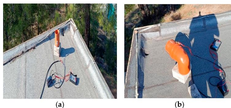
**Figure 12.** (a) Vertically polarized helical. (b) Horizontally polarized helical under test.
