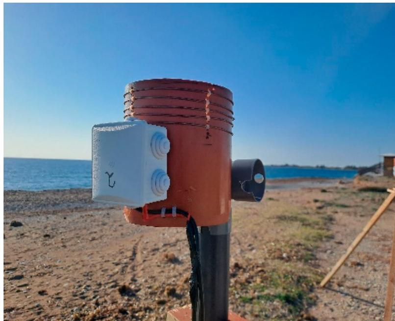
Figure 1. The normal-mode helical antenna under test.
