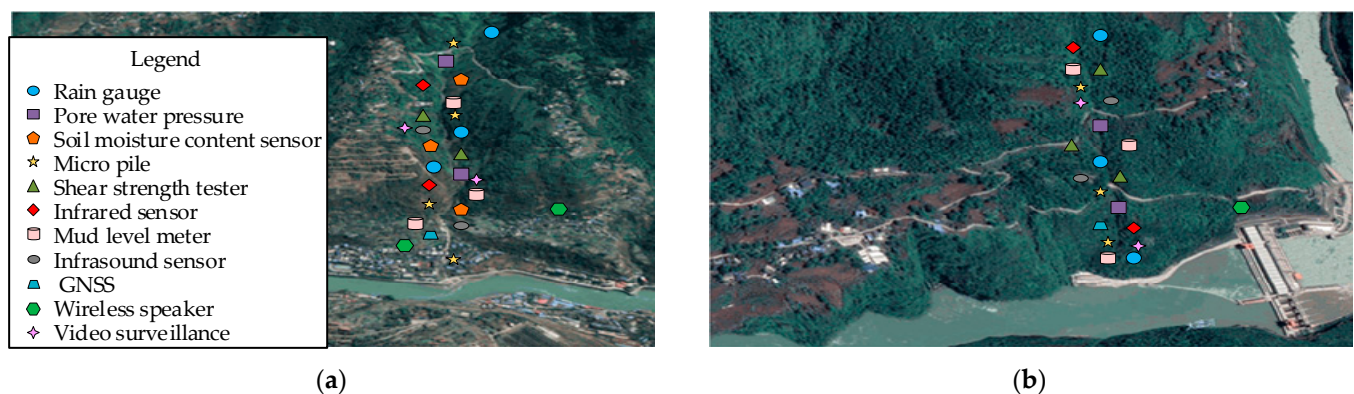
Figure 7. Layout of the monitoring sensor network. (a) Zhangcungou layout; (b) Longtan layout.
