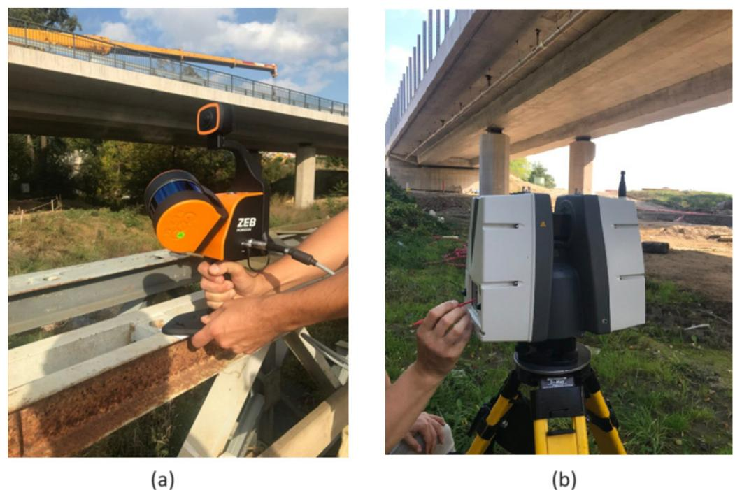
**Figure 2.** (a) Mobile laser scanner Zeb Horizon by GeoSLAM and (b) static laser scanner ScanStation P40 by Leica.
