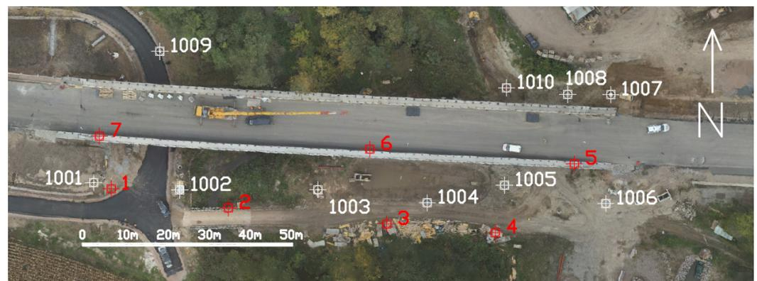
**Figure 3.** Overview of the (ground) control points. Here, 1–7 indicate vertical black and white targets serving as ground control points (GCPs) for the Leica P40 scanner (red), and 1001–1010 are horizontal targets used as GCPs for SLAM cloud transformation into the Czech coordinate systems (white).
