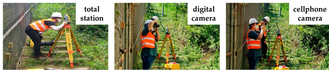
Figure 7. Field experiments with the traditional monitoring method (total station) and digital image photogrammetry (commercial imaging devices, digital camera, and cellphone camera).
